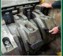
Segmented drum rotor with brute package has twenty striker plates held in place by two 1-1/4" bolts, designed for contaminated demolition debris, railroad ties, and MSW. Striker plates, edged with aggressive carbide, pulverize material and outlast with impressive durability, saving time and money. Striker plates pictured to the right.
