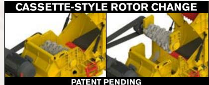
Adapt to changing demand patterns by swapping to a new rotor. Go from grinding to chipping in half the time.
