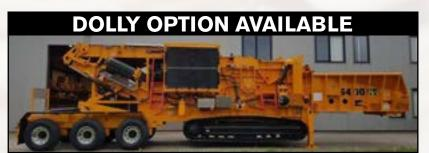
60" wide by15' long infeed. Side walls wing outwards to funnel material, reduce spillage, and allow more feeding clearance.
