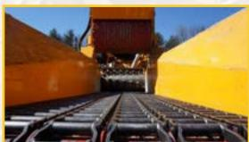
Infeed walls wing outwards to increase loading clearance and funnel material.
